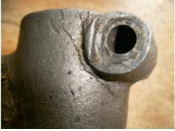
pulling himself over the cockpit side by grabbing the steering wheel. We'll never know how it got damaged, however, it has now been repaired and fitted to the car with an additional support block mounted inside the U of the chassis rail to take the strain from the brake pedal shaft. Just to complete the job in the steering department, I've invested in a new Ulster steering column clamp from the Seven Workshop to replace what I think was a column clamp off a Triumph Herald.
