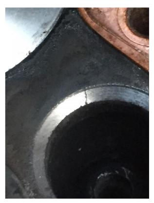
I am not sure if the valve caused the crack or the crack seized the valve - it extended into the block so I made the decision to remove it (in situ) and machine up another block to fit - I did this over the space of an evening, finishing by torchlight...
