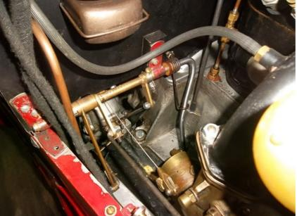
the steering box terminating in a manufactured cable end to suit the angle of the floor.
