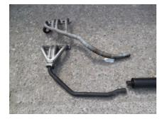
The new exhaust manifold and fabricated downpipe is now fitted as one piece and just sneaks through the gap between the front cross member and the full length undertray before bending upward to give enough clearance for the silencer to be fitted above the undertray. The old tail pipe had been made out of a modified box tailpipe passing over the axle but a pe-
