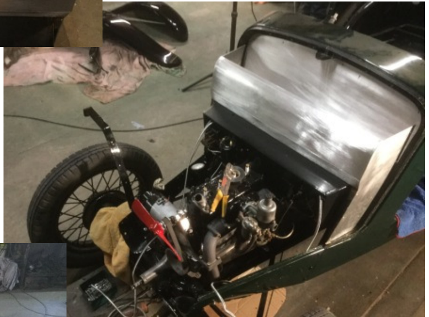
Another view of the bulkhead compartment being formed
