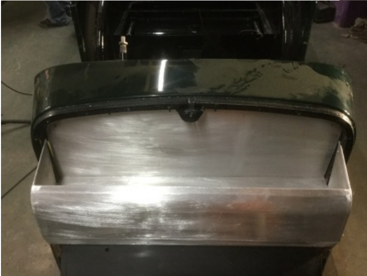
Bulkhead compartment being formed
